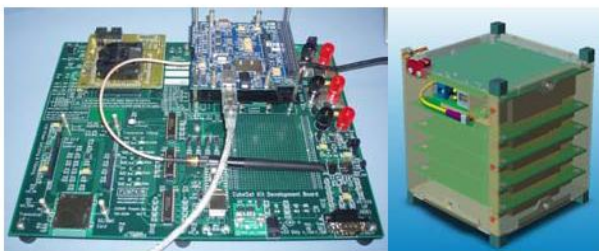
Figure 7. CubeSat development kit and the proposed picosatellite
